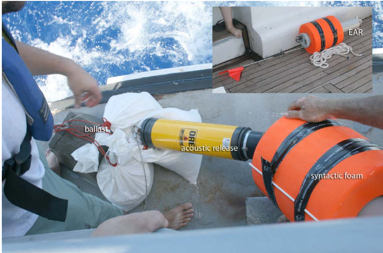
Figure 3.4-1: An EAR with the Components Labeled. The actual recording device is inside the tube surrounded by syntactic foam (see inset). This unit was deployed near Kaula Islet in June 2011.
