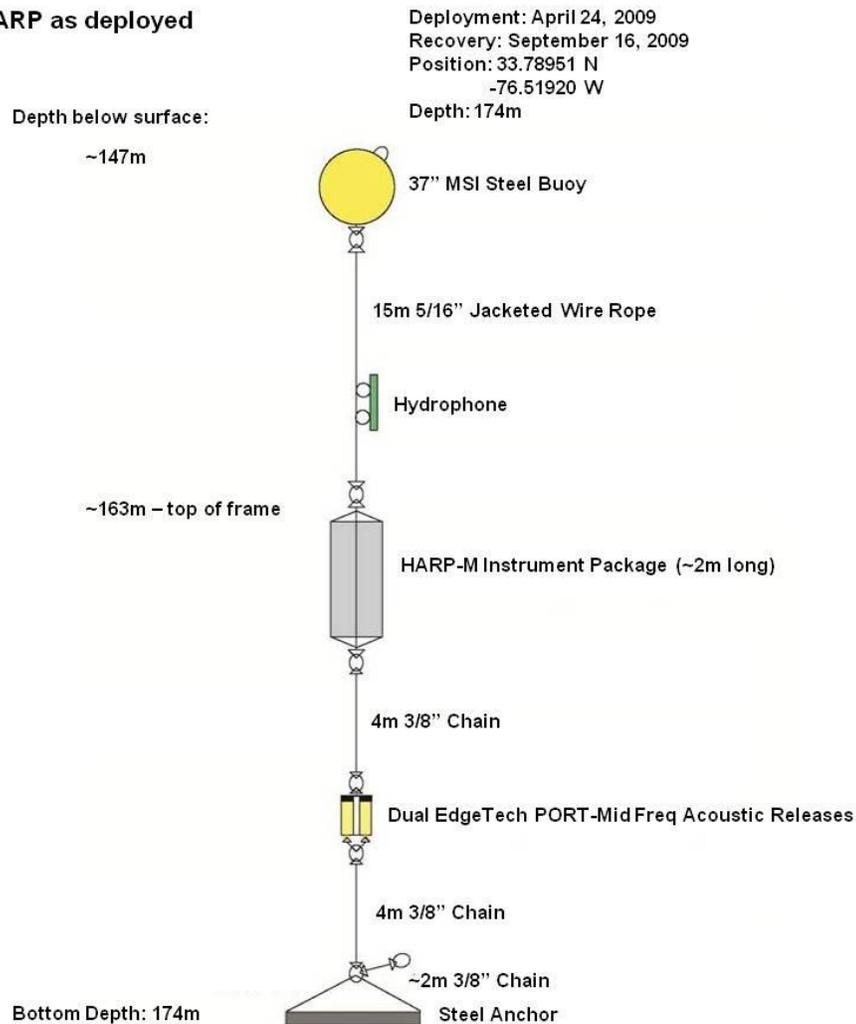
Figure 2. Schematic diagram showing details of the Onslow Bay 03A HARP. Note that diagram is not drawn to scale.
