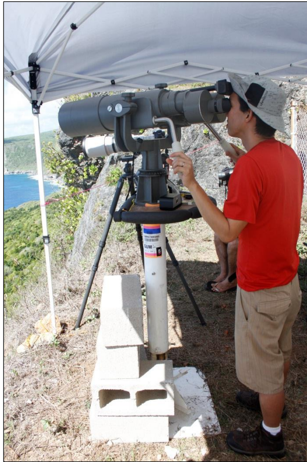
Figure 3. Big Eye binoculars with mounting stanchion stabilized with cinder blocks (photograph by J. Aschettino).
