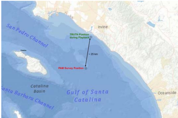
Figure 7. Example showing the PAM survey position (red) and playback vessel position (green) at the time of an acoustic detection of playback sonar. In this example playback sonar was detected at a distance of ~25 km.
