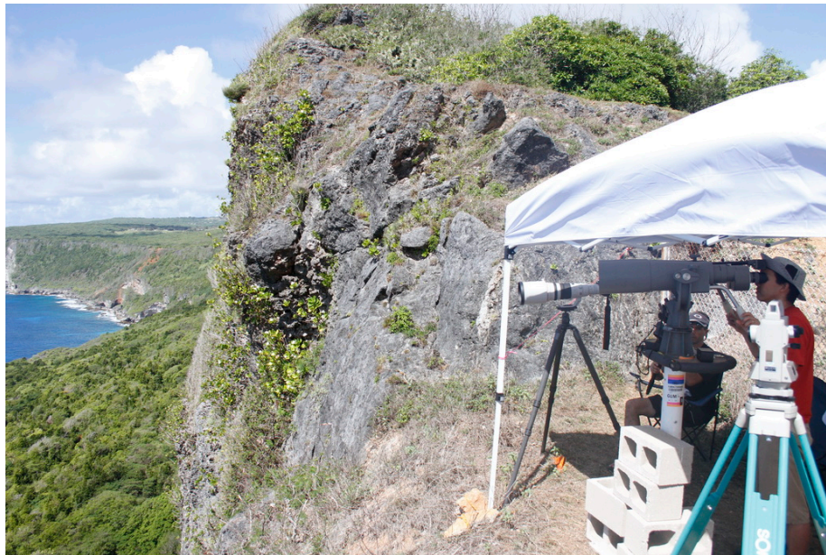
Figure 12. Shore station marine mammal survey on Guam utilizing Big Eye binoculars, theodolite, super-telephoto photography, and hand-held binoculars. (Deakos et al. 2014)
