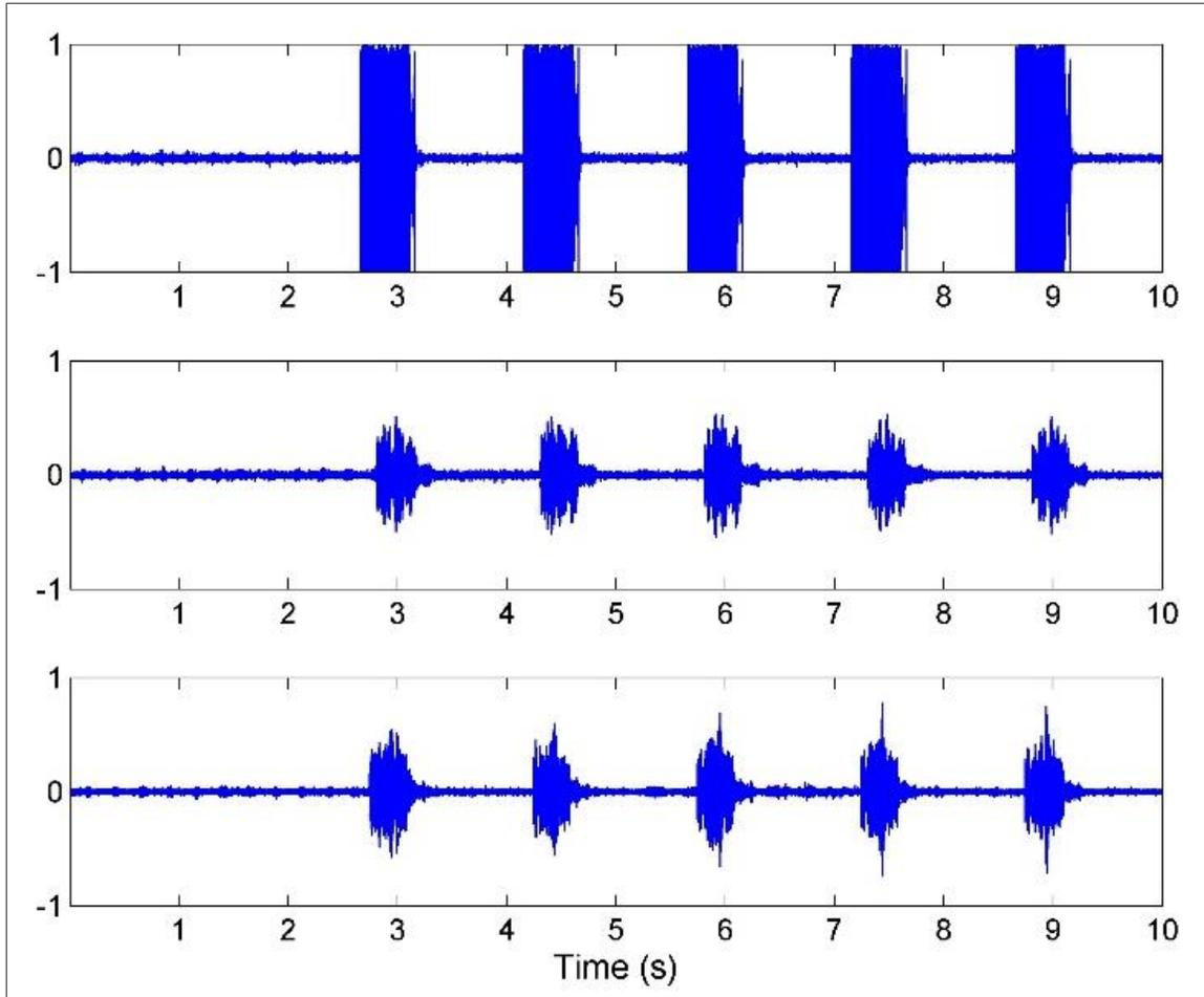
Figure 6. Example of the time-aligned pinger source signal as it was received at EAR B (top), Q (middle), and R (bottom). Y-axis values represent volts.
