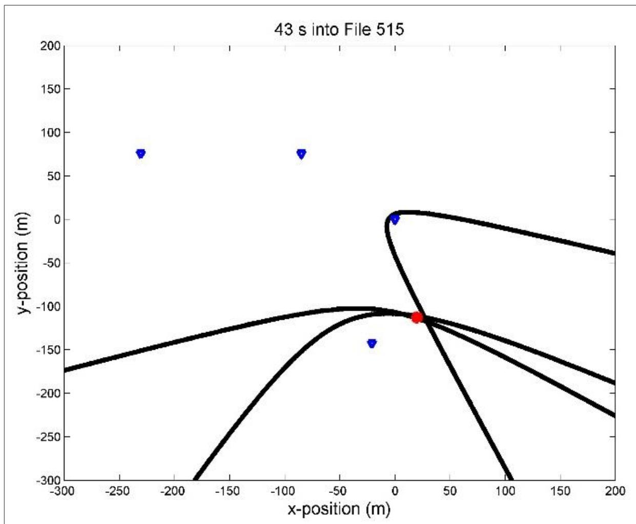
Figure 7. Example of a localized dolphin whistle. The blue marks indicate the positions of the four EARs. The red dot is the position of the signaling dolphin inferred by the convergence of the three hyperbolae.
