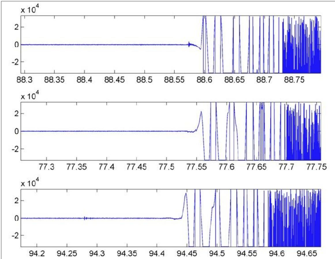
**Figure 5.** Zoomed-in view of low frequency precursor to the UNDET impulse on the three EARs. Note the phase inconsistency between the top panel and the two lower panels. The Y-axis represents 16 bit analog-to-digital sample values; the X-axis shows the time from the beginning of the recording at each EAR in seconds.
