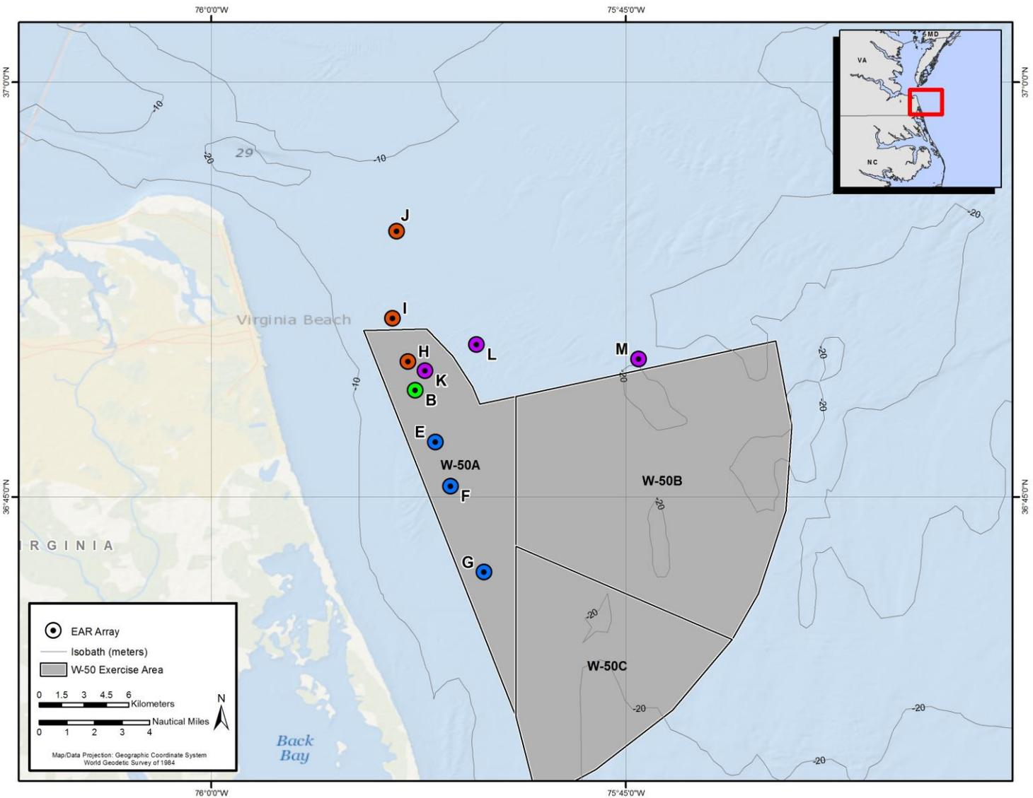
Figure 3. Spatial configuration of three linear coastal EAR arrays deployed during the second year of the project. Site B remained constant and north is shown as red (B–H–I–J), east as purple (B–K–L–M), and south as blue (B–E–F–G).
