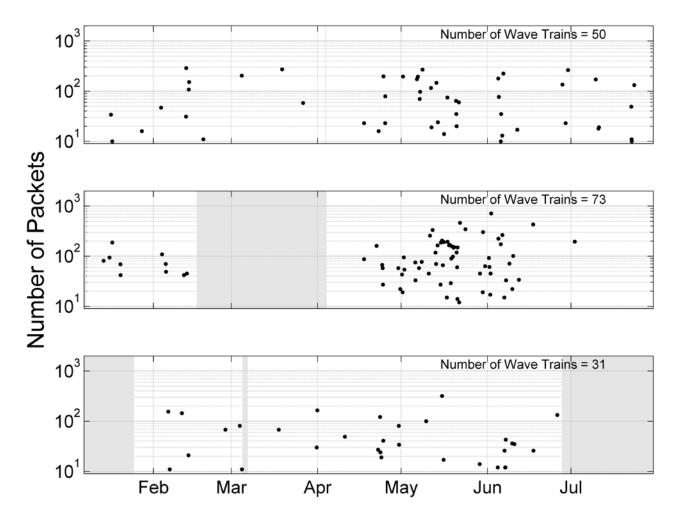
Figure 27. Number of MFA sonar packets for each wave train at sites H (top), N (middle), and P (bottom). Note the vertical axes are logarithmic base-10.
