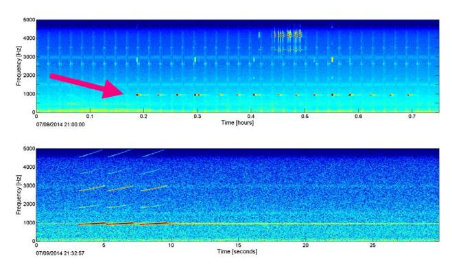
Figure 8. LFA at 950 Hz in the LTSA (top) and spectrogram (bottom) at site H.
