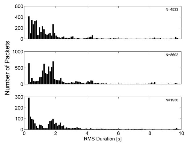
Figure 25. MFA sonar packet RMS duration distributions for sites H (top), N (middle), and P (bottom). The total number of packets detected is given in upper right corner of each panel. Note the vertical axes are at different scales.
