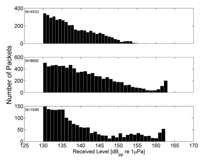
Figure 24. MFA sonar packet peak-to-peak received level distributions for sites H (top), N (middle), and P (bottom). The total number of packets detected at each site is given in the upper left corner of each panel. Note the vertical axes are at different scales.
