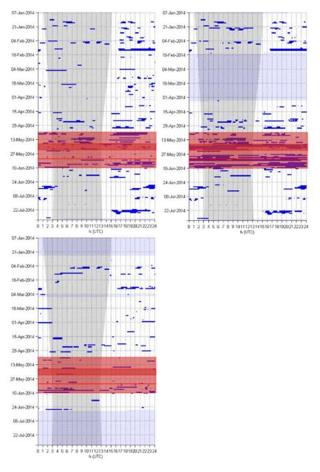
Figure 23. Major naval training events (shaded red) overlaid on MFA less than 5 kHz signals in one-minute bins at sites H (left), N (middle), and P (right). Effort markings are described in Figure 14.
